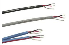
Industry standard balanced audio cable for permanent installation. Stranded tinned-copper conductors are easy to solder or punch-down. A high grade polyethylene dielectric is used to minimize high frequency attenuation, while excellent process control and tight pair twisting achieves superior noise rejection. Foil shield with same gage drain
