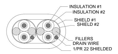
Description: 2/Pair 22 AWG Solid Tinned Copper, Dual Insulated, Each Pair Individually Dual Shielded
