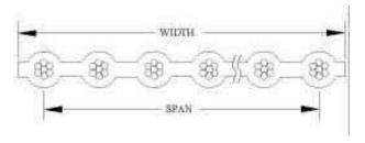
Conductors are 28 AWG silver plated copper. Conductor stranding is 7/36 and pitch is 1mm (0.0394 inches). Insulation is FEP extruded so that there are no de-lamination issues. Color is solid blue or blue with a blue polarity stripe. Packaging is 100 feet per reel, 50 feet minimum average length, 10 feet minimum length.
