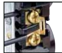
Back & Side Wiring Option of (1) side wiring or (2) back wiring: Insert wire into well. Tighten screw, thus clamping wire against terminal. Back wiring for copper or copper/clad aluminum conductors.
