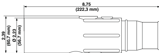
Male Plug – Double Set Screw Detachable
