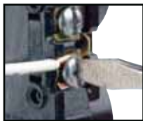
Side Wiring Loop wire around terminal screw. Screw head locks wire against terminal. For copper or copper/clad aluminum conductors.
