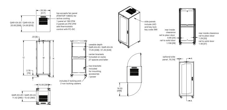
Note: side panels are required for door to lock/latch.
