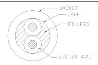
Product Specifications for 2/C 20 AWG 120 Ohm Unshielded Twinaxial Cable
