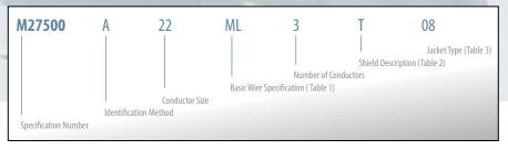
All the basic wire specifications listed below may be supplied by RSCC Aerospace & Defence as components in WC 27500 cables. These range from low temperature PVC/Nylon leads through high performance, high temperature constructions. The basic wire specification, part number designation symbol, and a brief description of the insulation type are listed in Table 1.
