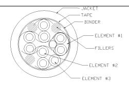
**Description:** 9/C composite cable consist of 1/Pairs 20 AWG shielded, 3/Pairs 20 AWG and 1/C 20 AWG, HD-PE Insulation, Overall Nylon tape and Polyurethane Jacket
