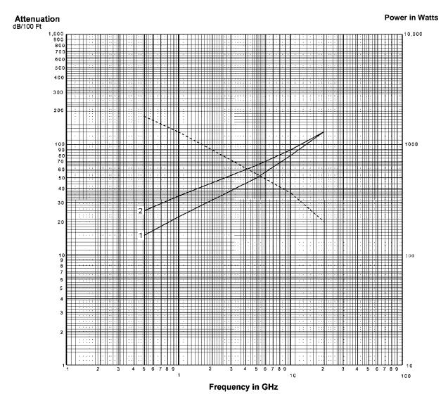
Maximum attenuation \_\_\_\_\_ (Test requirements shall be as noted as line indicated on graph.) Maximum power ------ At 25°C at sea level.
