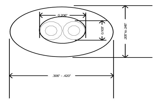
\*\*These are approximate dimensions. We will have exact dimensions upon completion of the prototype To hit exact dimensions at this time would require very expensive precision tooling
