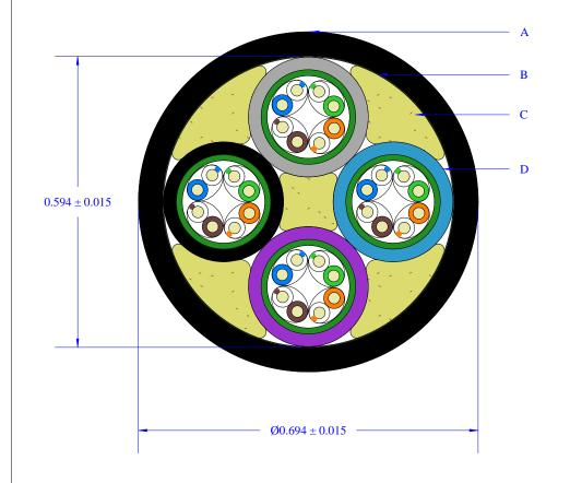
A: Thermoplastic Elastomer Jacket, Nominal Jacket Thickness: 0.050, Pressure Extruded, Color: Black, Temperature: -40°C to 80°C Non-UL
