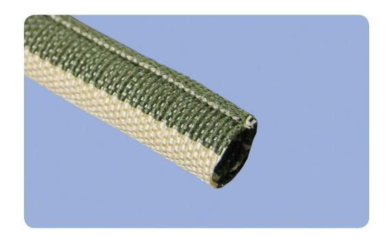
**ROUNDIT® 2000 NX HT** is a self-wrapping sleeve manufactured from PEEK monofilaments and Nomex® multifilaments. It includes an oil and water repellent treatment in order to prevent the absorption of condensation build-up caused by the extreme changes aircraft are subjected to. Designed for mechanical protection and maintenance of wire and cable bundles, its 100% covering ratio provides excellent cut-through and abrasion resistance.
