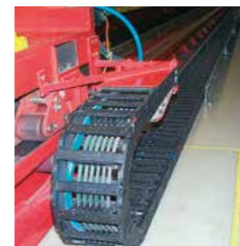
Chainflex® CF5/CF6 for storage retrieval unit: Long travel in longitudinal axis. E-Chain®: Series E4/00 with igus® guide trough made of steel
