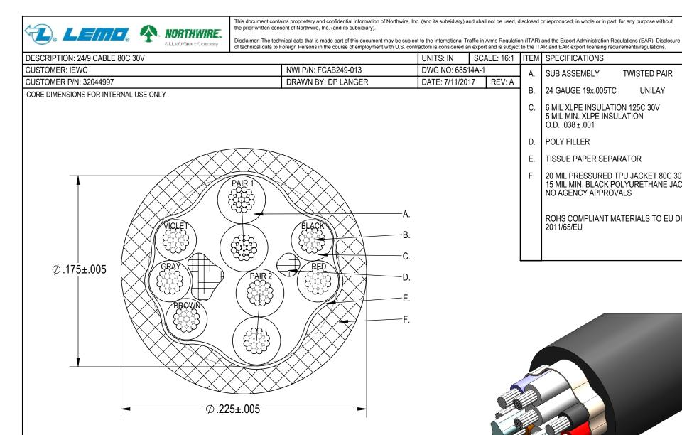
REV: A Β. 24 GAUGE 19x.005TC UNILAY 6 MIL XLPE INSULATION 125C 30V C. **5 MIL MIN. XLPE INSULATION** O.D. .038 ± .001 D. POLY FILLER E. TISSUE PAPER SEPARATOR F. 20 MIL PRESSURED TPU JACKET 80C 30V 15 MIL MIN. BLACK POLYURETHANE JACKET NO AGENCY APPROVALS ROHS COMPLIANT MATERIALS TO EU DIRECTIVE 2011/65/EU **ISOMETRIC VIEW** FOR REFERENCE ONLY
