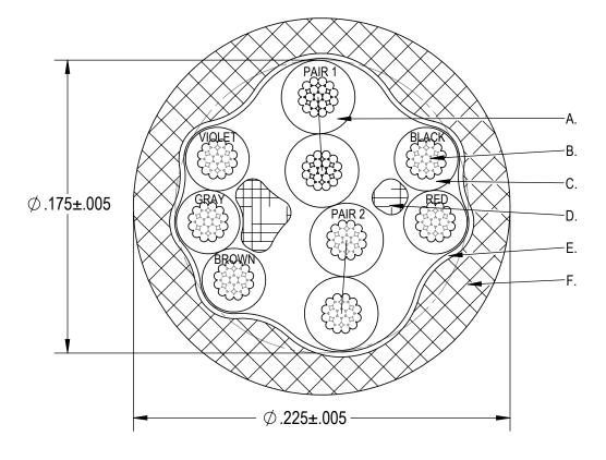
6 MIL TEFZEL (ETFE) INSULATION 125C 30V 5 MIL MIN. ETFE INSULATION O.D. .038 ± .001 D. POLY FILLER
