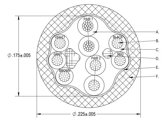
5 MIL MIN. XLPE INSULATION O.D. .038 ± .001 D. POLY FILLER TISSUE PAPER SEPARATOR F. | 20 MIL PRESSURED HYTREL JACKET 80C 30V 15 MIL MIN. BLACK POLYESTER HYTREL JACKET NO AGENCY APPROVALS ROHS COMPLIANT MATERIALS TO EU DIRECTIVE
