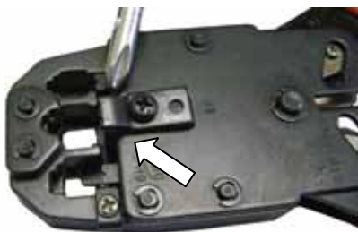
Image 3. Remove to prevent damage to the plug. Sku: 078-1017 (crimper)
