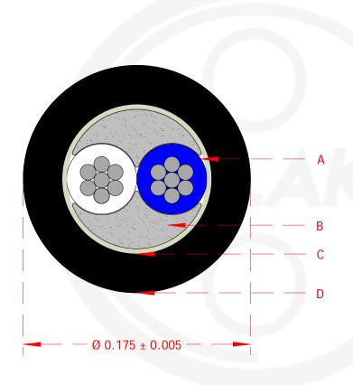
A: 20 AWG 2 Conductor PVC insulated Wire Size & Stranding: 20 AWG 7/0.0121 Metal Type: Annealed Tinned Copper Nominal Wire Diameter: 0.0363
