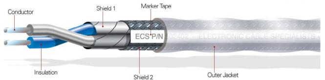
2 Conductors: 24 AWG silver plated copper alloy Insulation: High temperature flouropolymer Color Code: White, Blue Shield 1: Aluminum/Polyester foil Shield 2: 38 AWG tin plated copper braid Jacket: White high temperature flouropolymer (laser markable)
