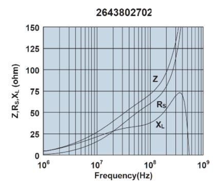
Impedance, reactance, and resistance vs. frequency.
