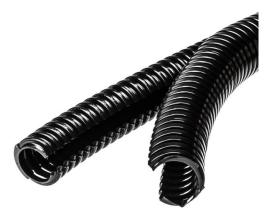
HelaGuard Non-Metallic Conduit, Double Slit, Std Wt, 0.50" Dia, Nylon PA6, Black, 164 ft/Std. Reel
