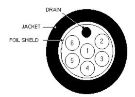
DESCRIPTION: SIX CONDUCTOR 20 AWG, HDPE, DRAIN & FOIL, BLACK PUR JACKET
