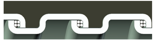
Square-Locked Design with cord packing 3/8" through 1-1/4"
