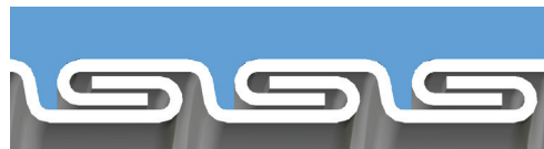
Interlocked Design 1-1/2" through 3" with no bonding wire
