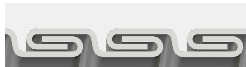
Interlocked Design 1-1/2" through 4" with no bonding wire
