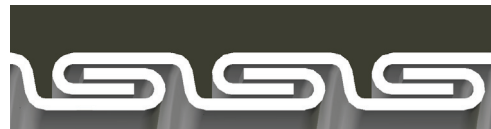
Interlocked Design 1-1/2" through 4" with no bonding wire
