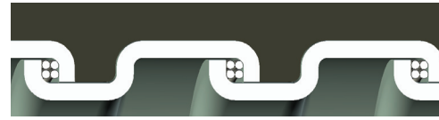
Square-Locked Design with cord packing 3/8" through 1-1/4"
