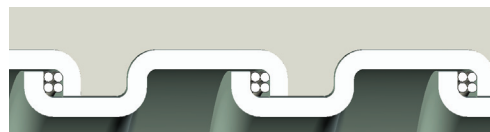
Square-Locked Design with cord packing 3/8" through 1-1/4"
