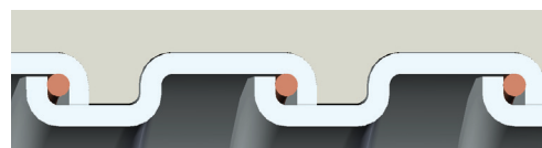
Square-Locked Design with integral bonding wire 3/8" through 1-1/4"
