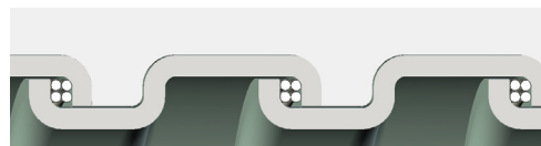
Square-Locked Design with cord packing 3/8" through 1-1/4"
