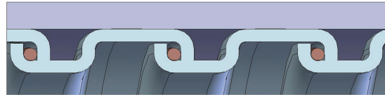
Square-Locked Design with integral bonding wire 1/2" through 1"
