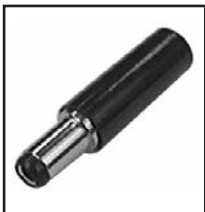
30-374 Bakelite Barrel 30-374-P With Strain Relief. Coax power plug. 2.5 mm I.D. 5.5 mm O.D. 9.5 mm long. .15" cable opening.
