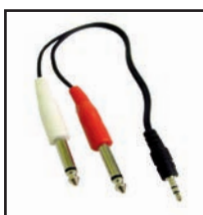
35-476 "Y" cable. 3.5mm stereo plug to dual 1/4" mono plugs, shielded. 10" long.
