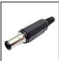
30-721 Sony DC power plug with plastic strain relief. 6mm O.D. Center pin 1.3mm 1.97 overall length. accepts .17" cable O.D.
