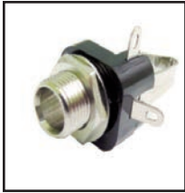
30-412A Closed Circuit 1/4" Mono Audio Jack. .35" x .29" bushing. .36" hole size, will work with standard .375" hole.
