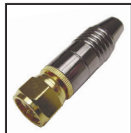
75-756 RG-6 High end solder type 'F' connector with black chrome plated barrel, gold plated 75 ohm connector with teflon insert. .32" cable opening.
