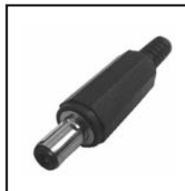
30-617-2.1 30-617-2.5 Locking DC power coax plug 5.5 O.D., 9.5mm long. Insert into 30-616 jack and twist clockwise to lock. .14" cable opening.
