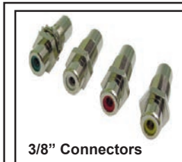
30-410-3/8-COLOR NICKEL 30-410G-3/8-COLOR GOLD Mounts in 3/8" hole. Bushing length .39" Overall length is 1.14".
