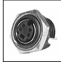
30-507 4 pin Japanese 30-507-T 4 pin Taiwanese 30-507-6 6 pin Taiwanese 30-507-8 8 pin Taiwanese 4, 6, & 8 pin chassis mount mini-din jacks. Mounts in 9/16" hole. Bushing length .167".
