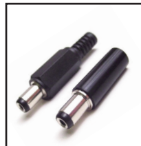
30-373 Bakelite Barrel 30-373-P With Strain Relief. Coax power plug. 2.1 mm I.D. 5.5 mm O.D. 9.5 mm long. .15" cable opening.
