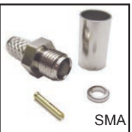
75-765 Female SMA 3 piece crimp connector for RG59/62. Nickel plated brass construction, gold plated contacts with teflon insulator.
