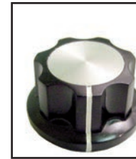
85-560 Black, bakelite knob. Fluted grip, \frac{1}{4} -inch brass bushing with set screw. \frac{3}{4} " Diameter, \frac{7}{16} " high.
