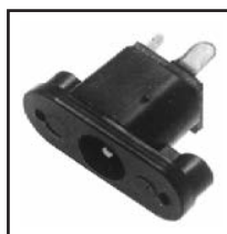
30-371 Coax power jack, standard chassis mount, 2.1mm pin. Switched circuit. 17mm mount center.
