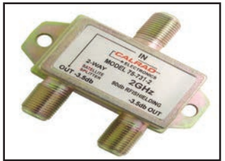
75-731-2, 2-WAY 2GHz, 90dB SATELLITE SPLITTER Power passive to all ports. Insertion loss 4-4.5dB max. Port-Port isolation 12-15dB min. Input return loss 12-15dB min. Zinc alloy die cast housing.
