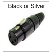
30-528-BK 30-528-SL XLR 3-pin Female plug, twist-on strain relief. .15" to .3" cable opening. Internal compression style cable strain relief.
