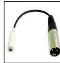
35-468 3.5mm stereo Female jack to XLR Male. Wired: pins 1&3 = ground pin 2 = tip 8" long with Black PVC jacket.
