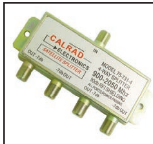
75-731-4 4 WAY 2GHz, 90dB SATELLITE SPLITTER Power passive to all ports. Insertion loss 6.7-11dB max. Port-Port isolation 11-15dB min. Input return loss 12-15dB min. Zinc alloy die cast housing.
