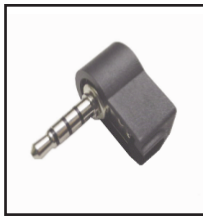
30-702 4 conductor 3.5mm right angle Audio & Video Plug. Tip, ring 1, ring 2, sleeve. Cable opening .14".
