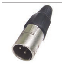
30-630-SL-3 3 pin 30-630-SL-4 4 pin 30-630-SL-5 5 pin Silver inline Male XLR plug. .15" to .3" cable opening. Internal compression style cable strain relief.
