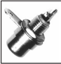
30-428-COLOR Nickel 30-428G-COLOR Gold Nickel plated RCA Audio Jack with hex nut and solder lug. Single hole mount. 1/4" hole. Bushing length .25" Available with black, blue, green, orange, red, white and yellow inserts.
