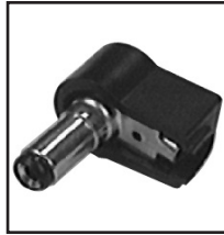
30-356 Right angle coax power plug. 2.1mm I.D., 5.5mm O.D. with solder terminals. .22" x .12" cable opening.
