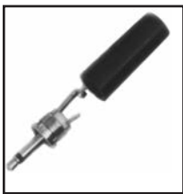
30-423A 2.5 mm sub-mini Audio Plug with plastic grip, 2 cond. Improved solder points. 7/16" plug length. .15" cable opening.
