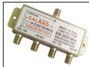
75-730-4, 4 WAY 2GHz, 90dB SATELLITE SPLITTER Power passive to one port. Insertion loss 6.6-9dB max. Port-Port isolation 11-23dB min. Input return loss 12-15dB min. Zinc alloy die cast housing.
