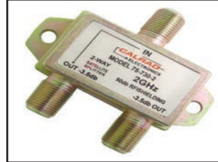
75-730-2, 2-WAY 2GHz, 90dB SATELLITE SPLITTER Power passive to one port. Insertion loss 3.4-5.5dB max. Port-Port isolation 11-15dB min. Input return loss 12-15dB min. Zinc alloy die cast housing.
