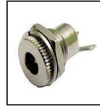
30-378 Japan 30-378-T Taiwan 2.5mm I.D. 5.5mm O.D. chassis mount coax power jack. For \frac{7}{16} " dia. hole in panels up to \frac{3}{16} " thick.
