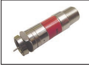
75-726 75 Ohm DC BLOCKER 5-1750MHz, insertion loss 0.3dB, return loss 16dB typical. Nickel plated machined brass. Passes RF and blocks DC from the signal path. Male 'F' connector to F-81 style female. Overall length 1.6".
