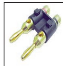
30-604-CT-BK 30-604-CT-RD Dual gold banana plugs with flexible body. For up to 8 gauge wire. .15" cable opening. 0.75" centers.
