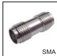
75-768 Female to Female SMA inline adapter. Nickel plated brass construction, gold plated contacts with teflon insulator.
