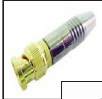
75-800G-75 75 ohm. RG-59 solder BNC connectors, gold with black chrome body. .255" cable opening.
