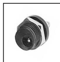
30-314 2.1mm I.D. X 5.5mm O.D. 30-315 2.5mm I.D. X 5.5mm O.D. Chassis mount coax power jack. Plastic housing. Mounts in 1/2" dia. hole. N/C switch.
