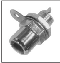
30-425-BK Black 30-425-RD Red RCA-type mini Audio Jack with hex nut grip, hex nut and solder lug. Single hole mount. 1/4" hole. 9mm hex base. Bushing length .27".
