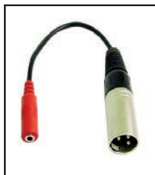
35-469 3.5mm stereo Female jack to XLR Male plug. Wired: pin 1 = ground pin 2 = tip pin 3 = ring. 8" long. Black PVC jacket.
