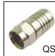
75-608S-RG59 75-608S-RG6 Quick one-step push on installation connectors suitable for coaxial broadband networks used in video and data. Precision machined annealed brass construction. Anti-corrosion nickel plated finish. Used with multiple cable braid and shield types. RG59 or RG6 standard, tri- shield and quad shield cable. Internal neoprene O-ring provides a weather sealed connection. 7mm heavy duty easy-grip nut.
