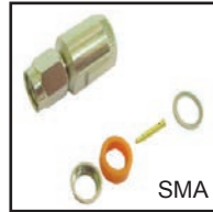
75-761 Male SMA connector for RG59/62. Nickel plated brass construction, gold plated contacts with teflon insulator.
