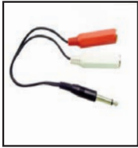
35-570 1/4" mono plug to two 1/4" mono jacks, shielded. 12" long.
