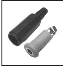
30-705 Inline Female 4 conductor 3.5mm Audio & Video Jack. Tip, ring 1, ring 2, sleeve. Plastic shell with strain relief. Mates to 30-700A, 30-701, and 30-702 plugs.
