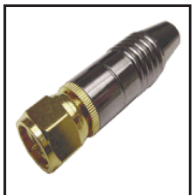
75-755 RG-59 High end solder type 'F' connector with black chrome plated barrel, gold plated 75 ohm connector with teflon insert. .255" cable opening.
