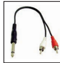
35-576 1/4" mono plug to two RCA Male plugs, shielded. 10" long.
