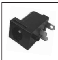
30-616-2.1 30-616-2.5 Locking DC power coax jack with N/C switch on sleeve side of the connector. Insert 30-617 plug and twist clockwise to lock.
