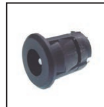
30-720-2.1 2.1mm version 30-720-2.5 2.5mm version Chassis mount snap-in coax power jack. Nickel plated connector with black molded trim. Mounts in .375" hole, up to .07" panel thickness
