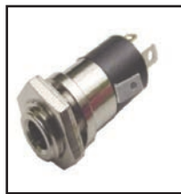
30-700A 4 conductor 3.5mm chassis mount stereo Audio & Video Jack. Tip, ring 1, ring 2, sleeve. Mounts in .28" hole.
