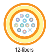
12-fibers Diagram scale approx. 3:1
