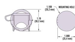
Nylon 6/6 Certifications Recognized under the Component Program of Underwriters' Laboratories File E15331 Ecertified by Canadian Standards Association File 8919 94V-2 Flammability Rating **Temperature Range** -.04°F (-18°C) to 221°F (105°C)
