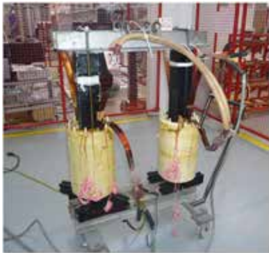
Two identical 75 kVA coils; One with 3M™ Insulation and one with calendared meta-aramid
