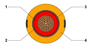
1 Core 4.0 mm<sup>2</sup> Type RADOX 155S FLR-B
