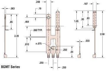
Alloy 260 Brass (70% Cu, 30% Zn. Higher Cu content resists dezincification) Tin-PI = Brass, Tin plated before or after stamping Post-Ni = Brass, Nickel plated after stamping **SN** Recognized Component under UL File E164169 Certified by the Canadian Standards Association File 91824 NEMA 1-15P & NEMA 5-15P
