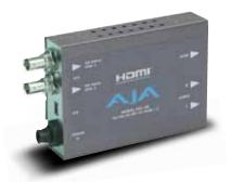
The Hi5-3G converts 3G-SDI, dual or single link HD-SDI, or SD-SDI to HDMI v1.3a for driving HDMI monitors. HDMI v1.3a capability at 30 bits per pixel allows full support of the latest 10 bit monitors. Audio is supported in the HDMI output allowing a convenient single cable audio/ video connection. The Hi5-3G provides 2 Channel RCA style audio outputs for separate audio monitoring if needed. USB connectivity allows for easy PC/Mac setup and field upgrades.
