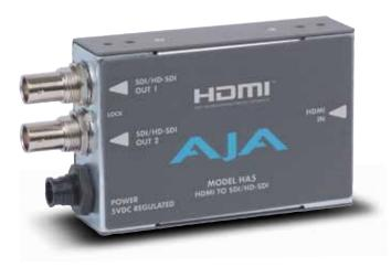
The HA5 converts HDMI to HD-SDI or SD-SDI in accordance with the input signal. Two channels of HDMI audio are embedded into the HD/SD-SDI output allowing a convenient single cable audio/video connection. The HA5 provides two HD/SD-SDI outputs and supports long HDMI cables on the input. The HA5 is useful for connecting HDMI cameras to HD/SD-SDI equipment.
