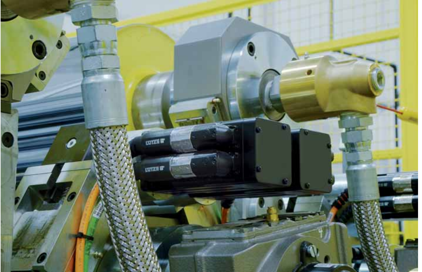
LUTZE Servo Cable Assemblies in action: Power- and Feedback assembly connected to motor jacks with SpeedTec connector!
