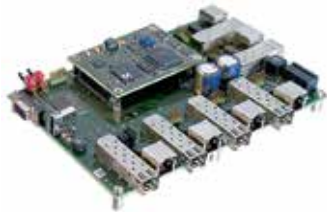
Example of Embedded Ethernet Switch EES25 on development kit
