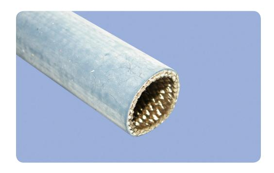
Ben-Har™ 1151-FRB Grade A is a rugged, flame-retardant, silicone rubber coated sleeving that provides excellent cut-through and abrasion protection for wiring systems in applications with temperatures ranging from -70°C to +200°C. Because the specially formulated silicone rubber is extrusion coated over the non-combustible fiberglass braid, it results in a reinforced sleeving that is superior to ordinary dip-coated sleeving and unreinforced rubber or plastic tubing.
