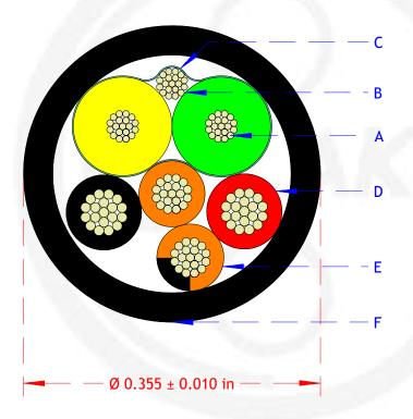
A: 20 AWG Shielded Twisted Pair 120 Ohm Can Bus
