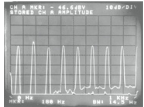
Fig. 2 Noise induced in two-conductor shielded cable (MVVS)
