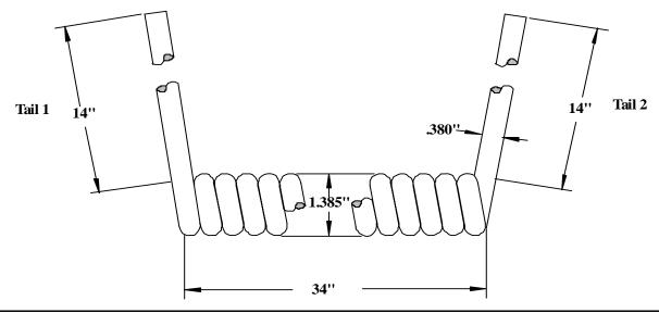
Three 18 AWG Insulated Conductors **Components**
