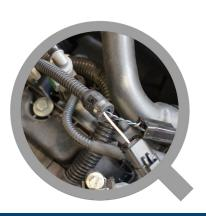
CLIPS are designed to maintain slit convoluted tubing closed.
