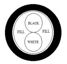
DESCRIPTION: TWO CONDUCTOR 16 AWG TPR INSULATION, FILLERS, CLEAR
