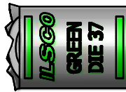
DETAIL A, SCALE 2 : 1 TOP INK MARKING INK COLOR: GREEN PER SPEC #: F921
