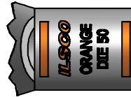
DETAIL A, SCALE 2 : 1 TOP INK MARKING INK COLOR: ORANGE PLT9 #115 HARDENER: PLH PER SPEC #: F921
