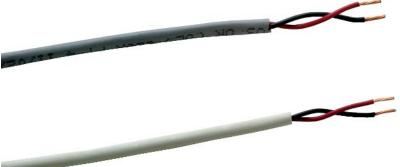
General purpose, economical audio and control cable for permanent installation in conduit, walls, or ceilings. The conductive elements consist of stranded, bare copper conductors that are insulated with a PVC insulation compound. The outer jacket is extruded from a 'ow-friction PVC that is easy to install and pull through conduit. Available in 20 and 22 gage types, each version is manufactured in both UL rated plenum or nonplenum constructions.
