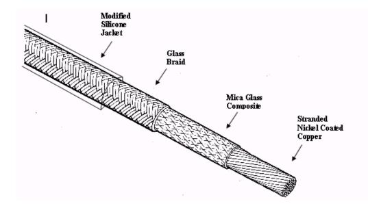
**DuraFlex®** 550s is the first UL listed 550°C AWM wire. The 550°C temperature rating allows wire to be used in extreme environments and reduces the costs of added thermal protection (glass sleeve, ceramic insulator, etc) to 450° C rated wire.
