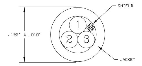
COMPONENTS - CONDUCTOR: #22AWG 19/34 TINNED COPPER (ITEMS 1-3) INSULATION: POLYRAD XT-. 016" NOMINAL WALL
