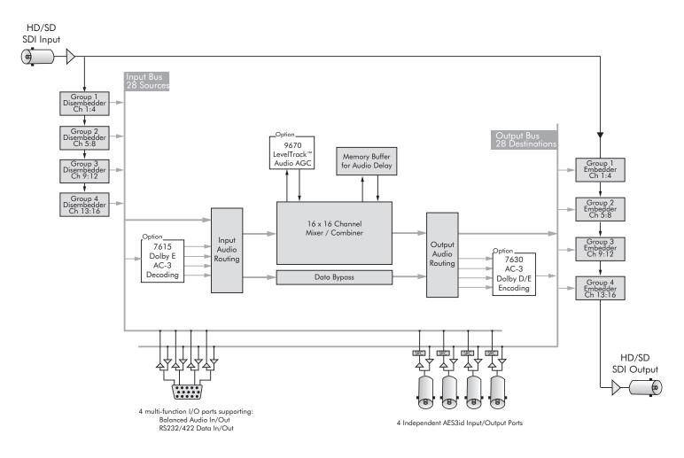
Above, block diagram for the 7660 HD/SD Embedder, Disembedder and Data Inserter module
