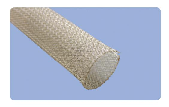
**Expando**® **686DM** is an expandable oversleeve designed for mechanical protection in temperature extremes and hostile environmental conditions. Rated to +200°C (+392°F), Expando 686DM meets VW-1 and FAR Part 25 flammability requirements.
