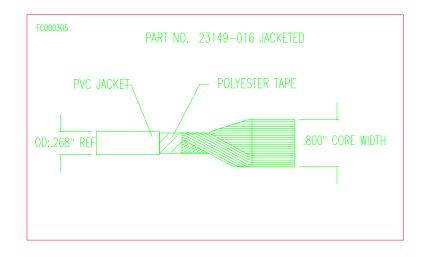
MARKING:THE CABLE IS IDENTIFIED WITH THE FOLLOWING PRINT LEGEND:<br/>HCM 23149 (UL) TYPE CM c(UL) 28 AWG 105C - Z/YY (XXXX)<br/>WHERE:MARKING:Y = YEAR OF MFG.<br/>YY = YEAR OF MFG.<br/>XXXX = JOB NUMBERAGENCY APPROVALS:UNDERWRITERS LABORATORIES, INC. TYPE CM CLASSIFIED<br/>COMMUNICATIONS CABLE FOR GENERAL PURPOSE COMMUNI-
