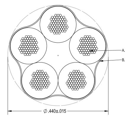
A. PURCAHSED SIS CONDUCTORS FROM IEWC 12 AWG 65x30TC 30 MIL INSULATION
