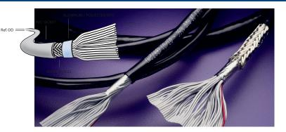
PHYSICAL CONSTRUCTION DESCRIPTION Cable core consists of slit and bonded flat gray ribbon cable. Core is folded and twisted into a round format before being taped with either Polyester (23149) or Aluminum/Polyester (23122) tape (Al side out). For dual shielded versions, cable is then braided. The core is jacketed in Black PVC.\*
