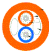
OUTER JACKET SUB-UNIT JACKET ARAMID STRENGTH ELEMENTS STRENGTH MEMBERS TIGHT BUFFERED FIBER
