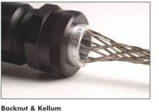
The included standard backnut features wrench flats and custom-sized gland seals that ensure a proper fit and weather resistance. In addition, the backnut can accommodate an optional kellem cord-grip for added strain relief.
